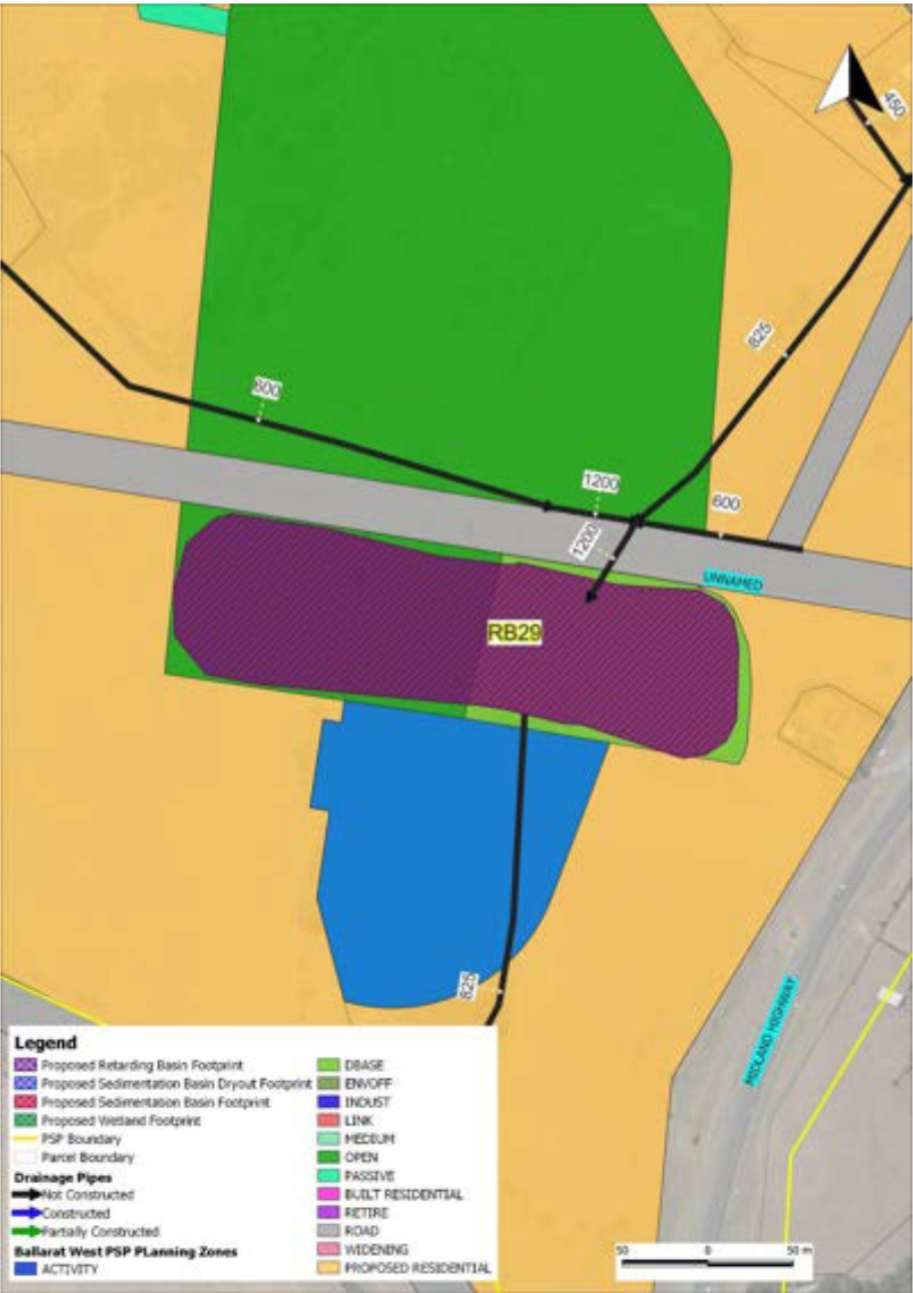
FIGURE 3.23: RETARDING BASIN 29 CONCEPT LAYOUT
