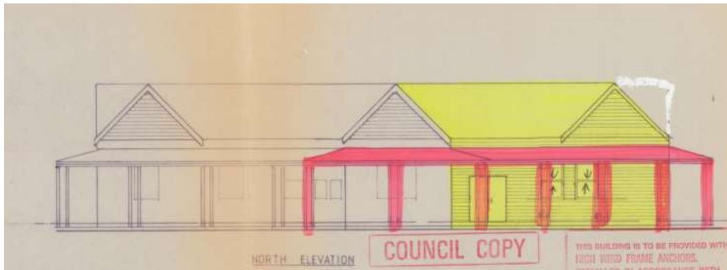
Figure 13. North elevation of Mossmont, with the western extension highlighted in yellow and the new parts of the verandah in red. Reproduction bargeboards were installed on the two western (right-hand) gables. (Shire of Buninyong, Building Approval No. 4977)
