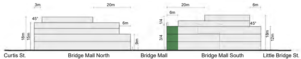
Figure 49 Built form test of street wall, setback and upper level heights- Section B
