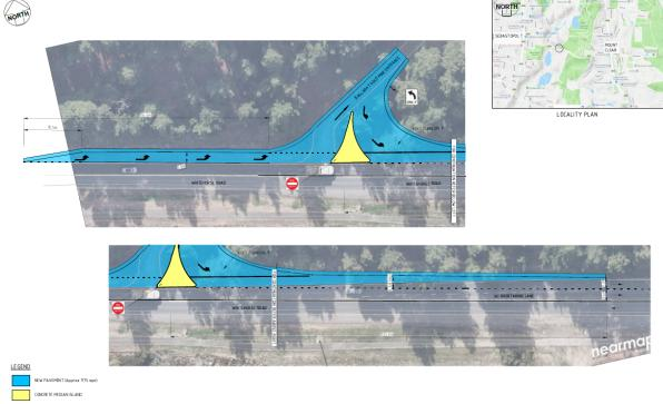
Figure 10 – Proposed access and road works (Source: Application)
