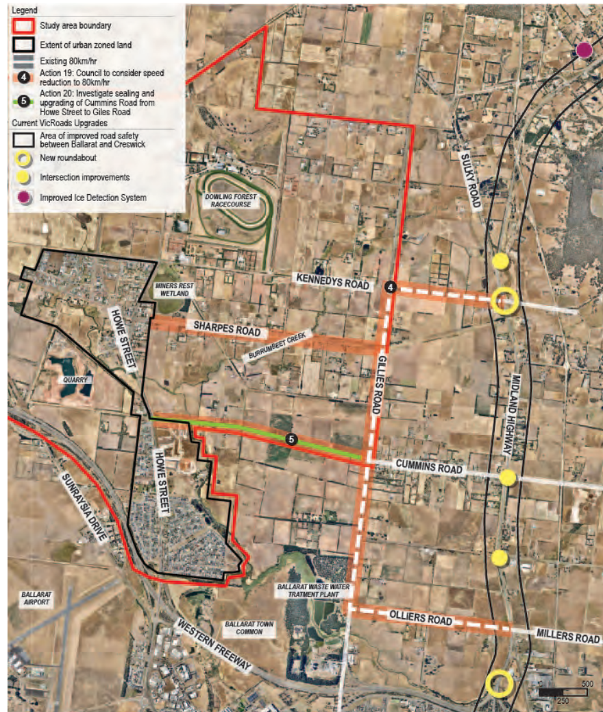
Action: Investigate reducing nominated traffic speed on Gillies Road, Kennedys Road and Olliers Road to 80km/h. Action: Seal and upgrading Cummins Road from Howe Street to Gillies Road
