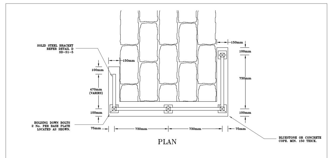
INSPECT EACH SITE PRIOR TO BARRIER FABRICATION AS CONDITIONS MAY VARY WITH REGARD TO DIMENSIONS &/OR ATTACHMENT DETAILS.
