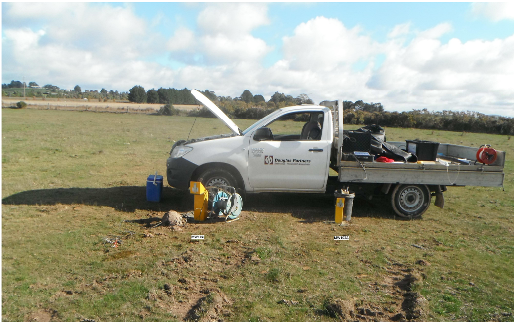
Photo 4 – Groundwater monitoring and sampling of boreholes MW102 and MW102A.
