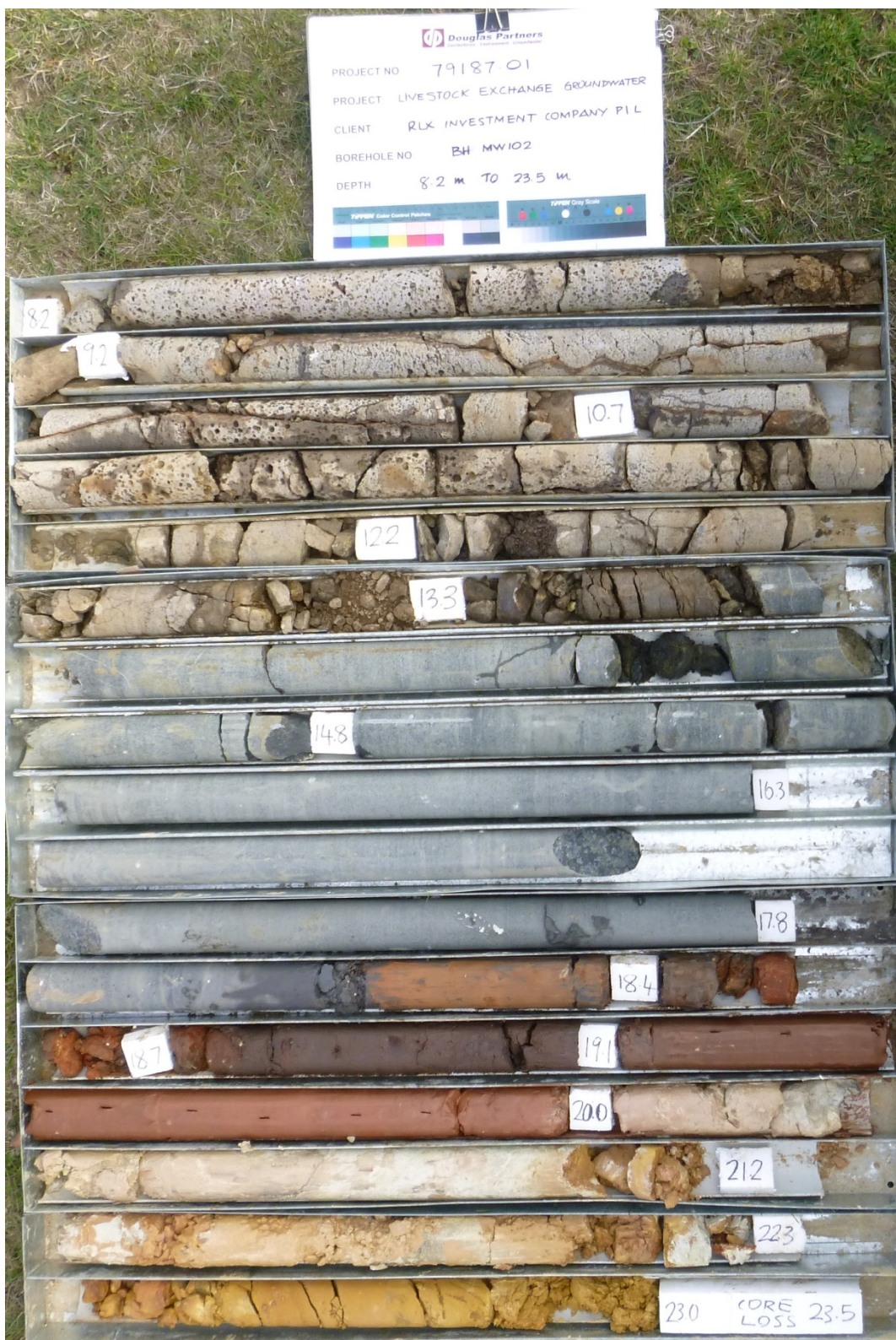
Core Photo 2: MW102, 8.2 m to 23.5 m.
