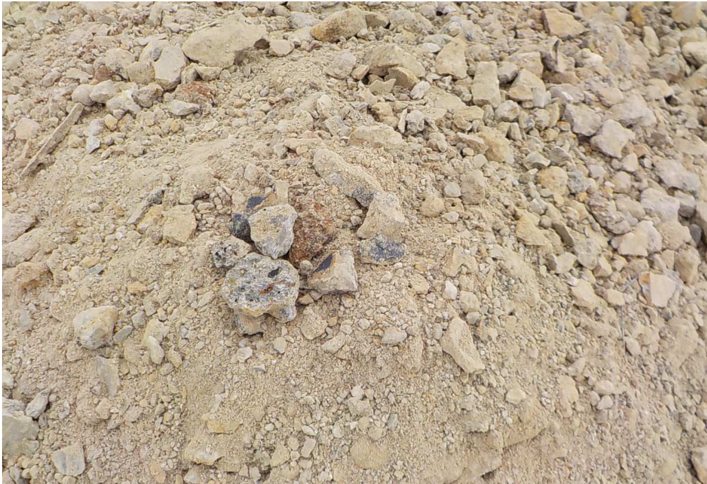
Photo 3 – Excavated spoil from TP121 showing basalt fragments.
