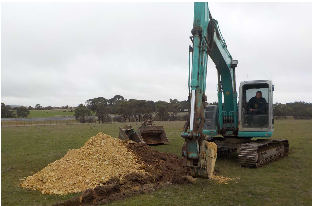
Photo 2 – Excavating test pit TP103, showing siltstone fragments.
