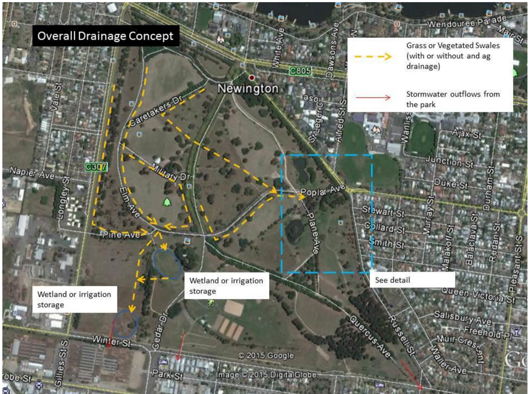
Figure 4: Potential network of swales to improve the overall drainage of Victoria Park.
