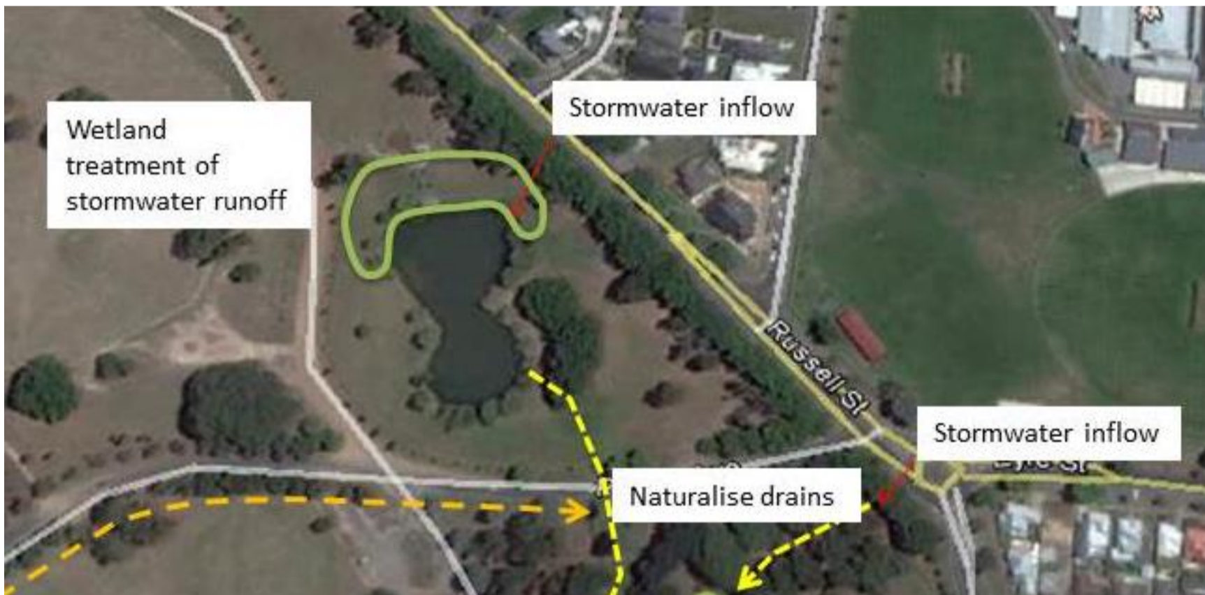
Figure 3: Schematic with a green outline (not to scale) illustrating the wetland proposed to remove pollutants from the St Leger catchment.
