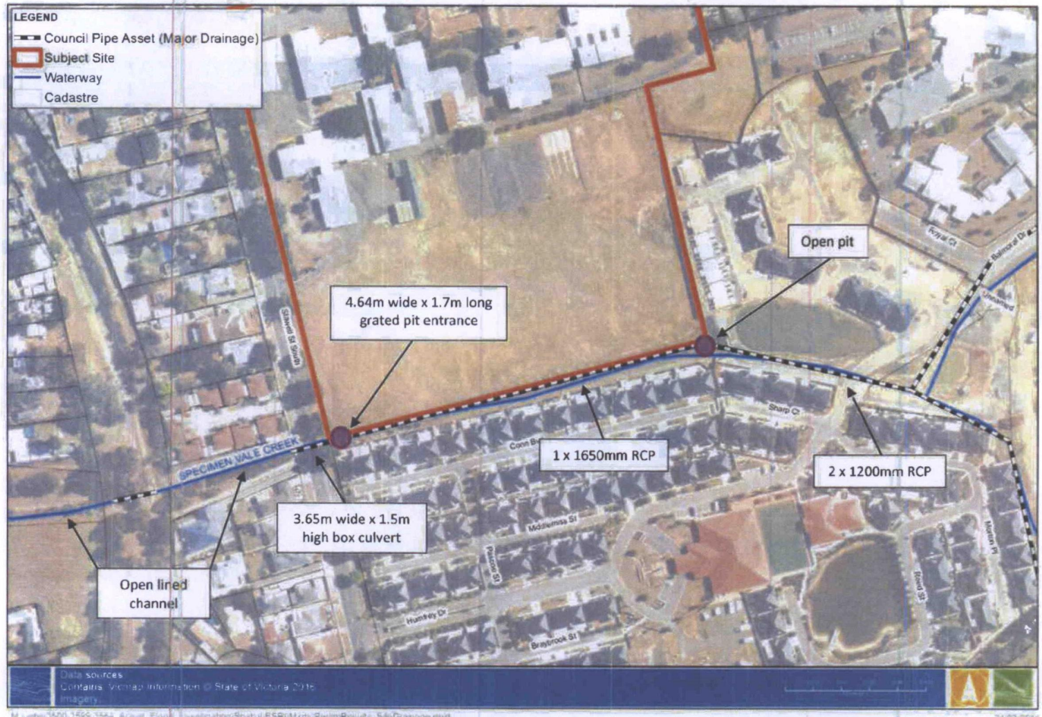
Figure 2-3 Drainage Features under Existing Conditions
