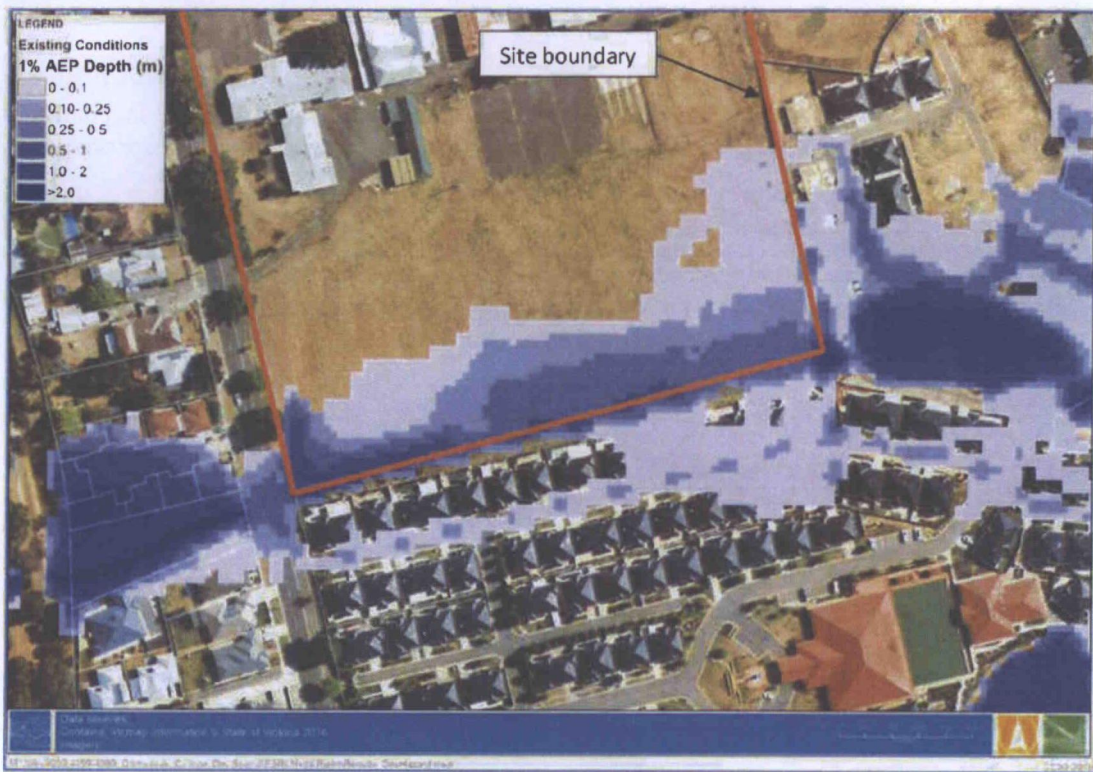
Figure 4-1 1% AEP flood depths under existing conditions
