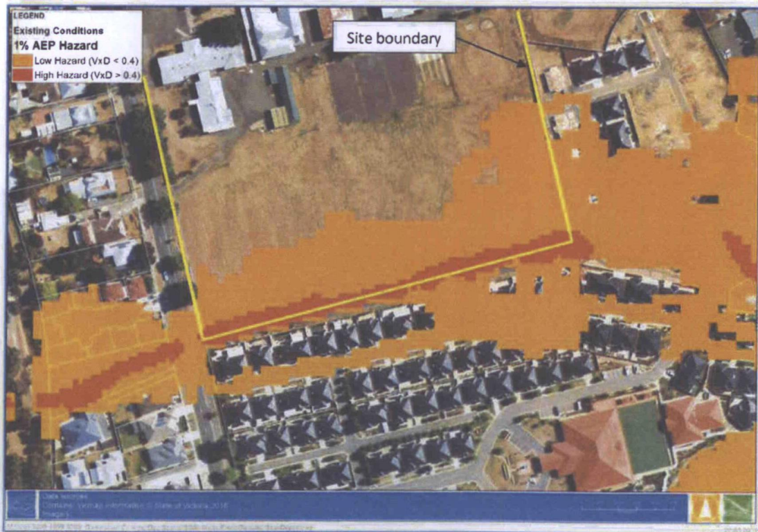
Figure 4-2 1% AEP flood hazard under existing conditions
