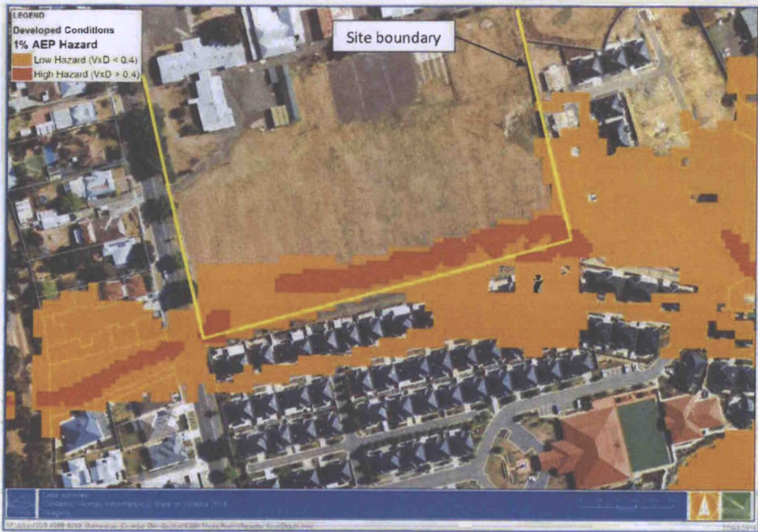
Figure 5-6 1% AEP flood hazard under developed conditions
