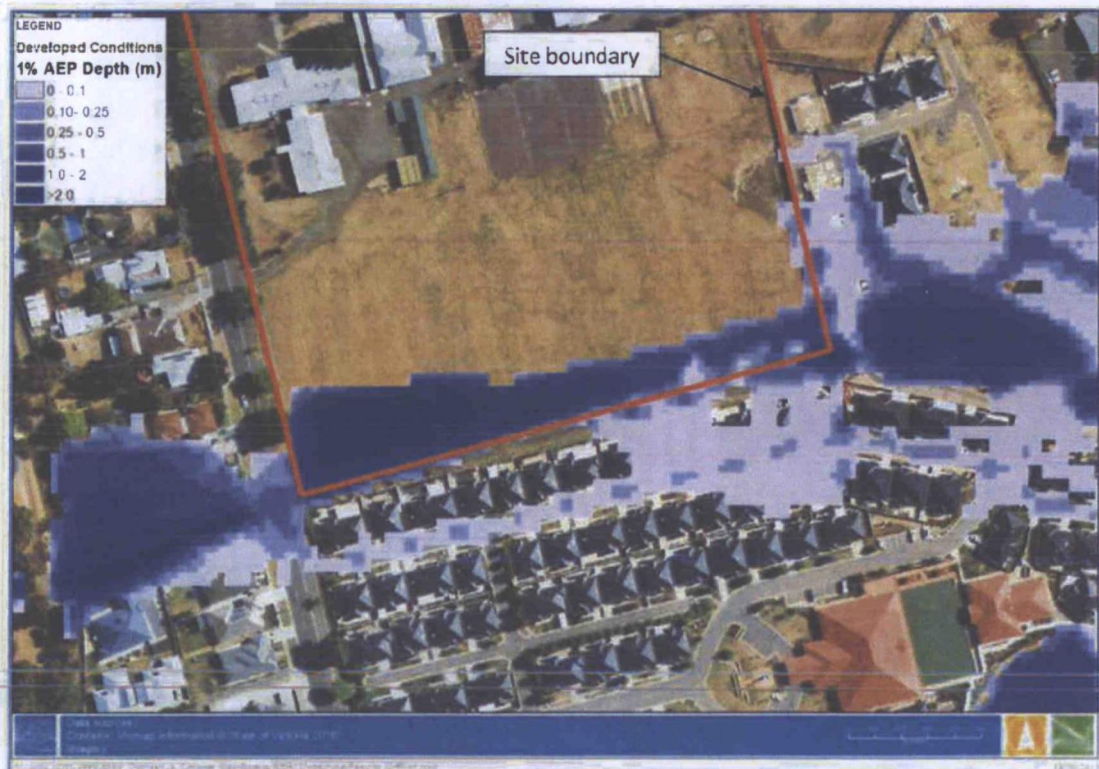
Figure 5-5 1% AEP flood depths under developed conditions
